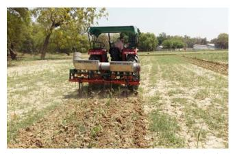
Fig. 5.3. Multipurpose tool frame with interculturing attachments
