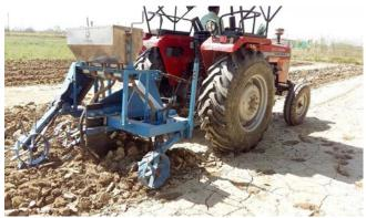
Fig. 5.7. Pant-ICAR sub-soiler cum differential rate fertilizer applicator in operation
