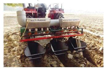
Fig. 5.2. Multipurpose tool frame with furrow opening attachments
