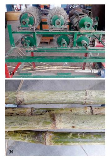
Fig. 6.1. Sugarcane cleaner-cum-washer (a) Cleaning unit, (b) Cleaned canes
