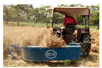
Fig. 5.8. Tractor operated reaper binder in field operation for wheat harvesting
