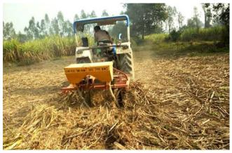
Fig.5.5. Two row disc RMD with stubble shaving attachment
