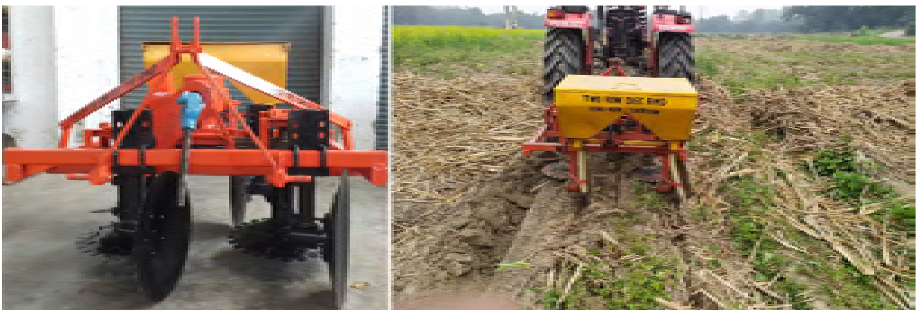
Fig. 5.1. Two row disc RMD with stubble shaving attachment
