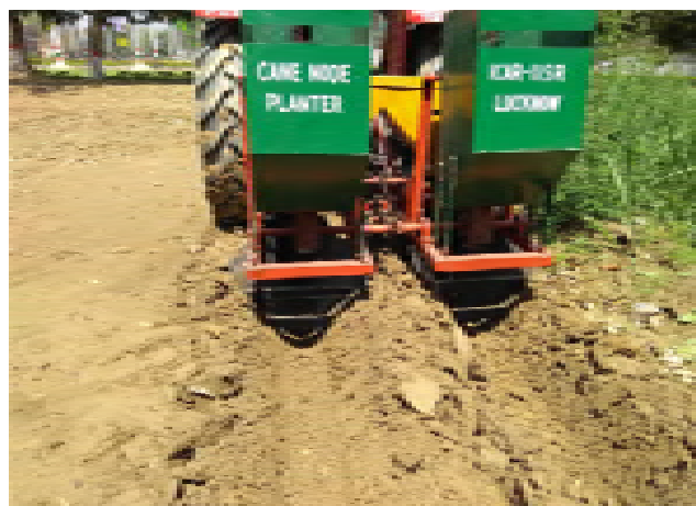
Fig. 5.6. Tractor operated cane node planter in field operation
