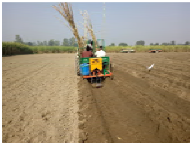
Fig. 10.4. IISR sugarcane trench planter in field operation at farmers' field
