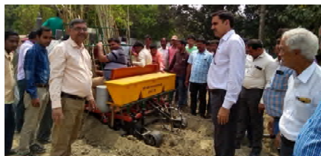
Fig. 10.7. IISR Tractor Operated Deep Furrow Sugarcane Cutter Planter-cum-Multicrop Raised Bed Seeder in field operation in Manpur, Sitapur
