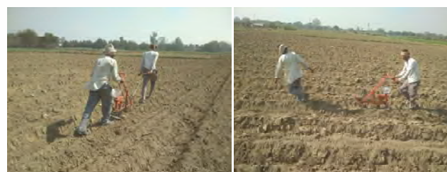
Fig. 5.13. Operation of Manual Multicrop Planter at IISR Farm
