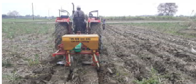
Fig. 5.2. Two row Disc RMD with stubble shaving attachment
