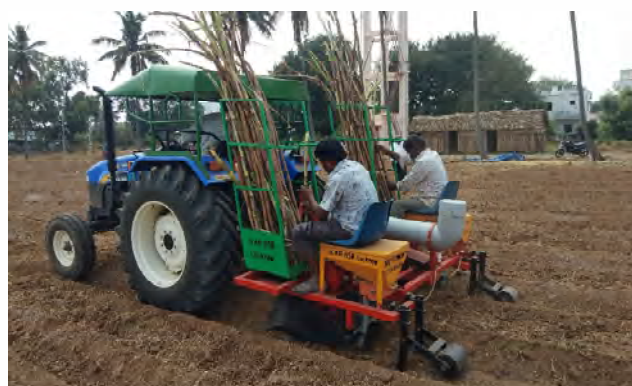
Fig. 5.9. Planting with IISR - Two row deep furrow sugarcane cutter planter in field at ICAR-SBI, Coimbatore farm
