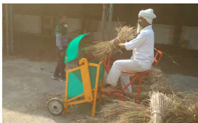
Fig. 5.15. Evaluation of the pedal operated paddy thresher
