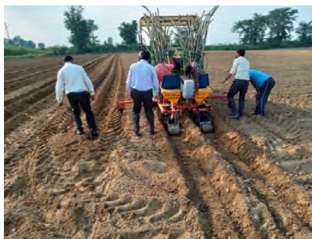
Fig. 10.5. IISR tractor operated modified deep furrow sugarcane planter in field operation
