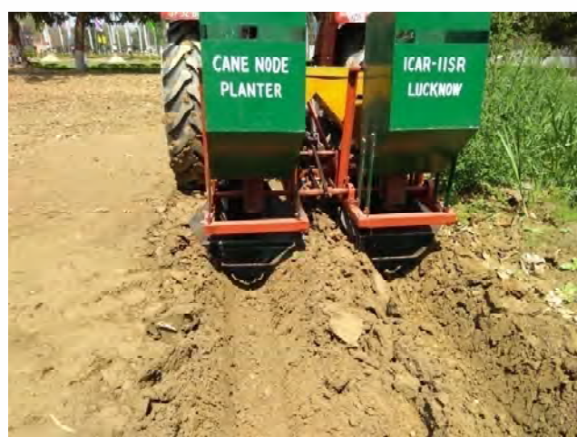
Fig. 5.4. Tractor operated cane node planter in field operation
