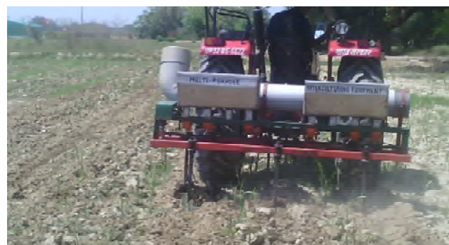
Fig. 10.8. IISR Tractor operated multipurpose interculturing equipment in field operation
