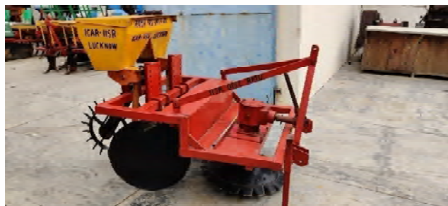
Fig. 5.10. Developed prototype of tractor operated disc type ratoon management device (Disc RMD)
