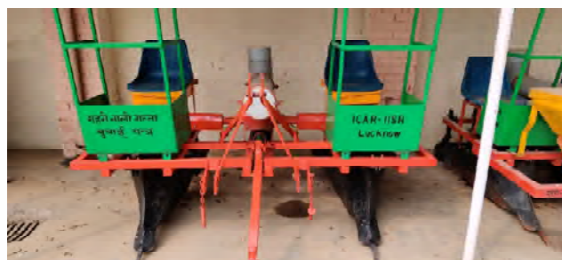
Fig. 5.8. Developed prototype of tractor operated wide spaced deep furrow sugarcane cutter planter
