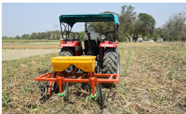
Fig. 5.1. Two row Disc RMD without stubble shaving attachment
