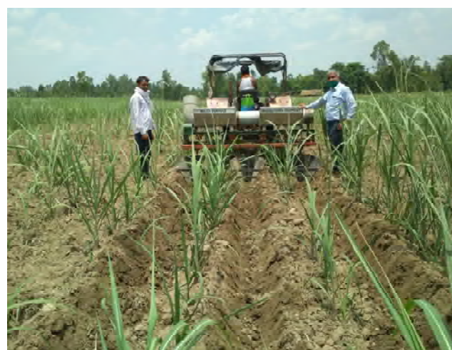
Fig. 10.9. IISR multipurpose interculturing equipment during earthing up mode
