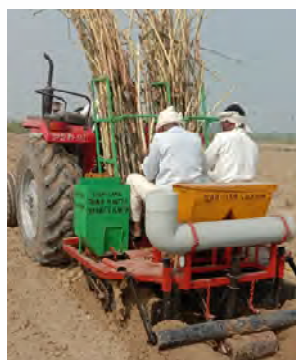
Fig. 5.16. Automatic potato-cum-sugarcane trench planter under field operation
