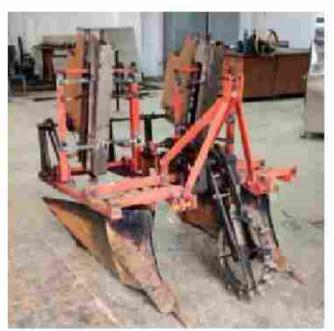
Fig. 5.1 Tractor operated cane node planter with modified cane metering mechanism
