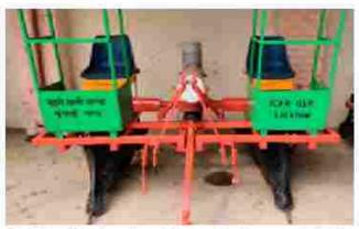
Fig. 5.6 Developed prototype of tractor operated wide spaced deep furrow sugarcane cutter planter
