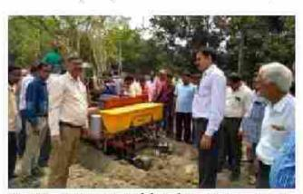
Fig. 10.7. Tractor operated deep furrow sugarcane cutter planter-cum-multicrop raised bed seeder
