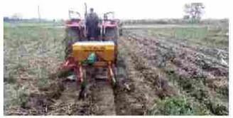
Fig. 10.6. IISR tractor operated two row disc type ration management device in field operation
