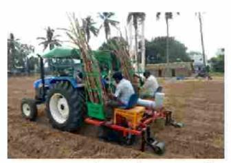
Fig. 5.7 Sugarcane planting with IISR - two row deep furrowcutterplanter at ICAR-SB1, Coimb atore farm
