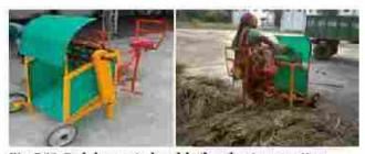
Fig. 5.11. Pedal operated paddy thresher in operation
