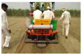
Fig. 5.10. Automatic potato-cum-sugarcane trench planter under field operation
