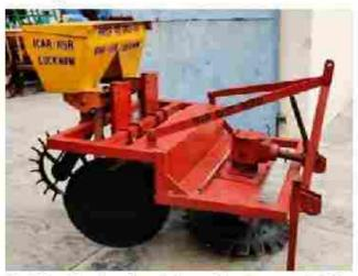
Fig. 5.8 Developed prototype of tractor operated disc typeratoon management device (Disc RMD)
