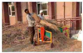
Fig. 5.17 Testing of motor operated paddy thresher
