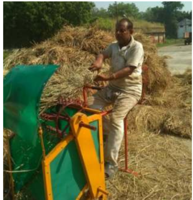
Fig.5.14 Pedal operated paddy thresher in operation
