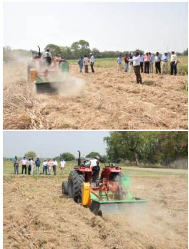
Fig. 5.2 Testing of tractor-operated trash mulcher-cum-stubble shaver device
