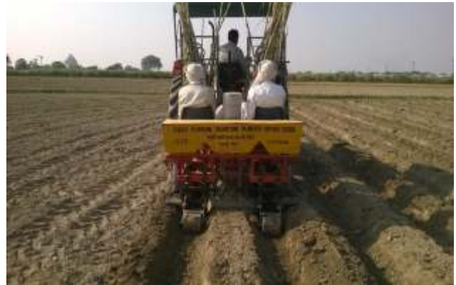
Fig. 10.3 IISR Tractor Operated Deep Furrow Sugarcane Cutter Planter -Cum- Multicrop Raised Bed Seeder in field operation
