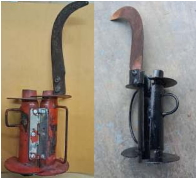
Fig. 5.3 Newly developed manual sugarcane stripper-cum-detopper
