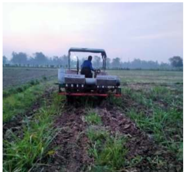
Fig. 10.4 IISR Tractor operated multipurpose interculturing equipment in field operation
