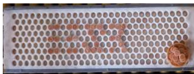
Fig. 6.5 Nylon Moulds for automatic moulding machine
