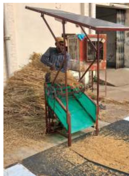
Fig. 5.15 Solar powered manual paddy thresher
