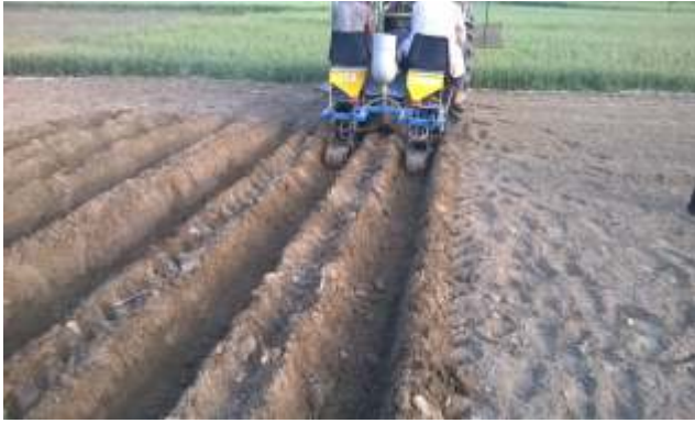
Fig. 10.1 IISR tractor operated modified deep furrow sugarcane planter in field operation
