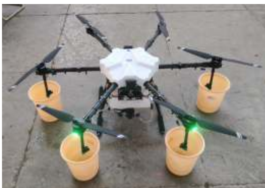
Fig. 5.6 Preliminary testing of drone for spray rate and nozzle volume at laboratory.
