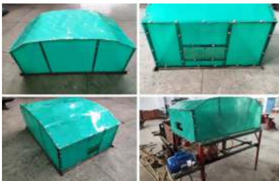
Fig. 6.1 Safety/protective cover provided on sugarcane cleaner-cum-washer
