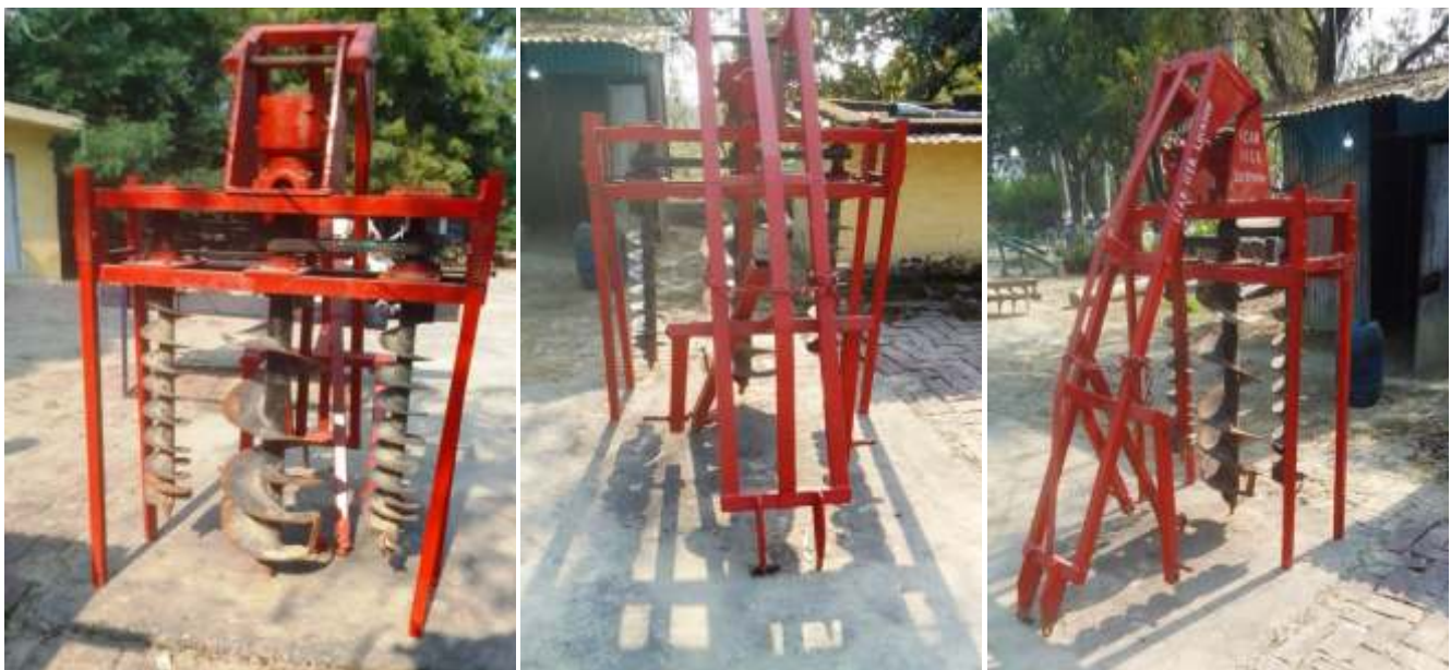
Fig. 5.8 First prototype of Multiple Auger System (MAS)
