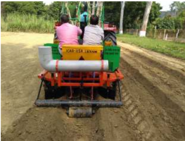
Fig. 5.13 Automatic potato-cum-sugarcane trench planter under field operation
