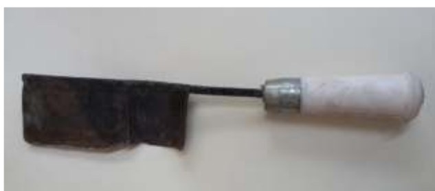
Fig. 10.6 IISR manual sugarcane stripper-cum- detopper
