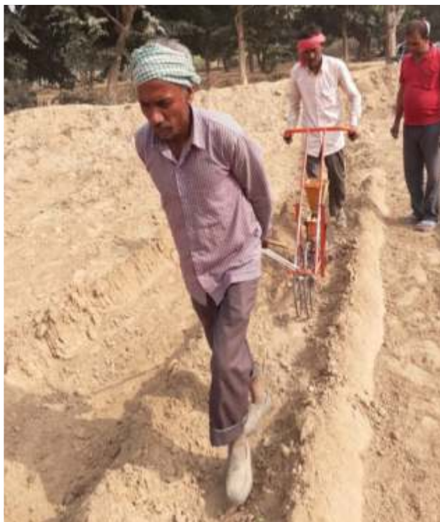
Fig. 10.5 IISR manual multicrop planter
