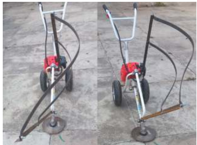
Fig. 5.17 Development of small harvesting system for sugarcane
