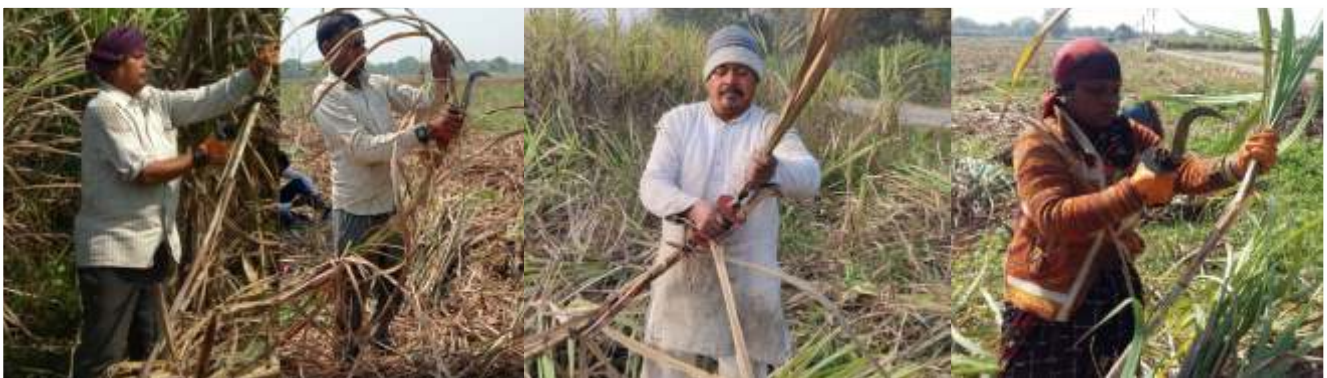
Fig. 5.4 Testing of newly developed manual sugarcane stripper-cum-detopper
