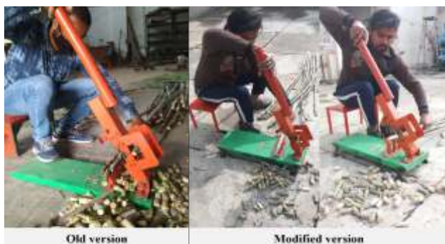
Fig. 5.5 Manual sugarcane seed sett cutting machine
