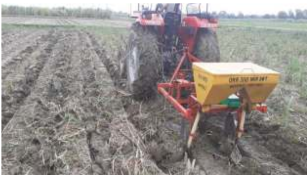
Fig. 10.2 IISR tractor operated two row disc type ratoon management device in field operation
