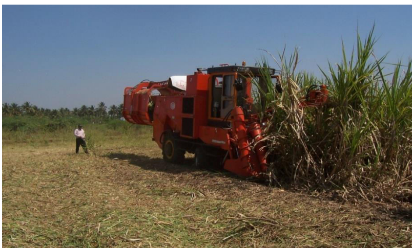
Fig. 4 Self propelled whole stalk cane harvester imported from China in field operation at Sathy (Tamilnadu)
