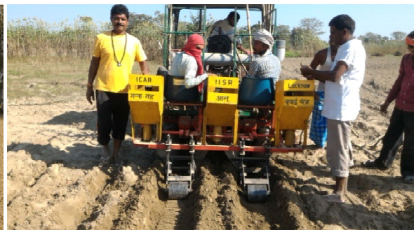
Fig. 8. IISR sugarcane-cum-potato planter
