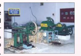
juice extraction, one should wash rollers and juice pipe line with hot water or steam to avoid microbial contamination.
