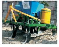
sharp edged concave spinning disc. The earthing unit provides soil cover over the stubbles in form of a ridge. This device place FYM and fertilizers simultaneously, adjacent to cane rows and dispense liquid chemicals in the soil gravitationally. An acre of ratoon field can be covered in about 1-1.5 hours as against 6 hours, if done manually.
