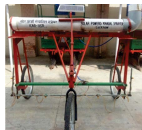
Fig. 6. Solar powered manual sprayer
