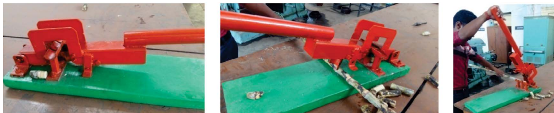
Fig. 1. IISR manual cane node/bud chip/sett cutting machine
