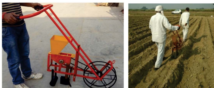
Fig. 3. Manual multicrop planter for sowing intercrop in sugarcane
